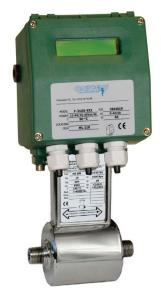
Faraday's Law states that a voltage will be induced in a conductor (the conductive fluid) when it passes through a magnetic field (generated by the meter) and that voltage will be directly proportional to the velocity of the conductor (the fluid). This voltage is measured by electrodes on opposite sides of the flow tube and used to calculate the flow velocity.
