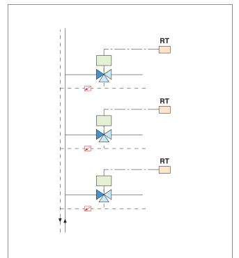
To guarantee the design flow rates (with open or closed valve) to the various zones of a system.
