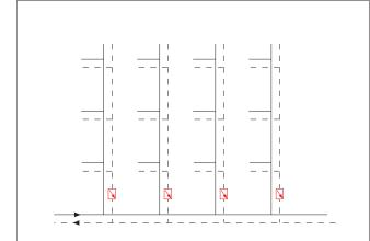
To regulate the flow rate in each riser or secondary branch of a system.
