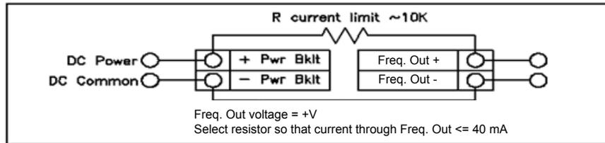
Figure 22. Non-Isolated Frequency Output Using External Power Supply
