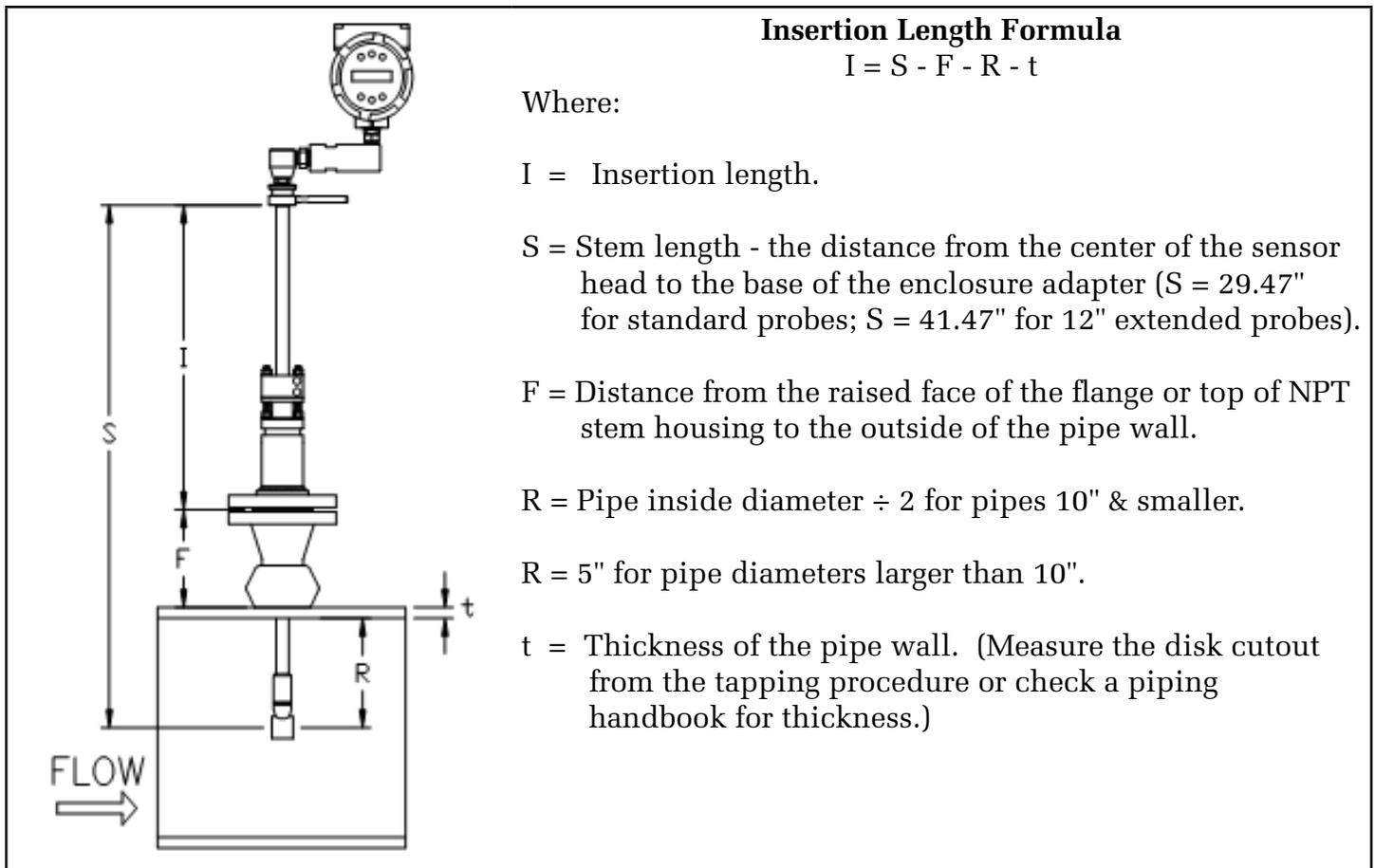
Figure 13. Insertion Calculation (Meters without Insertion Tool)
