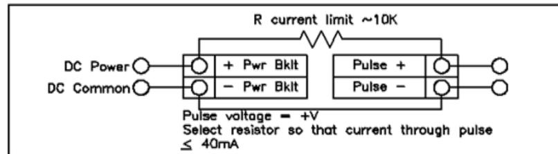
Figure 20. Non-Isolated Pulse Output Using External Power Supply
