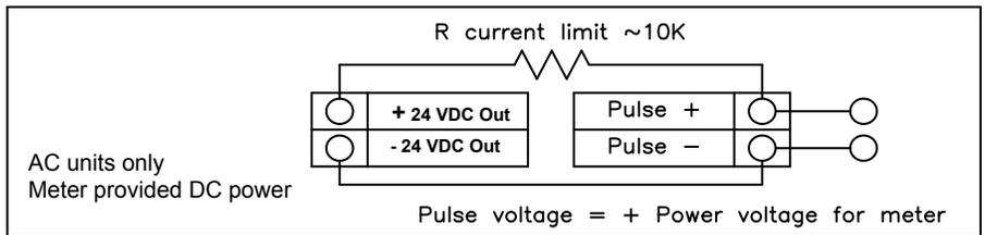
Figure 39. Isolated Pulse Output Using Meter Provided Power Supply
