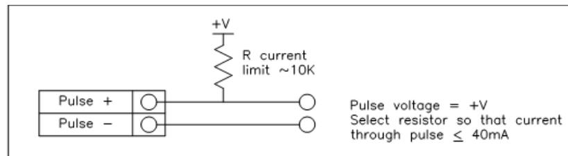
Figure 19. Isolated Pulse Output Using External Power Supply
