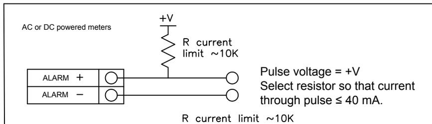
Figure 40 Isolated Alarm Output Using External Power Supply
