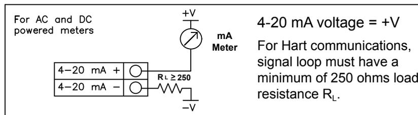
Figure 31. Isolated 4-20 mA Output Using External Power Supply
