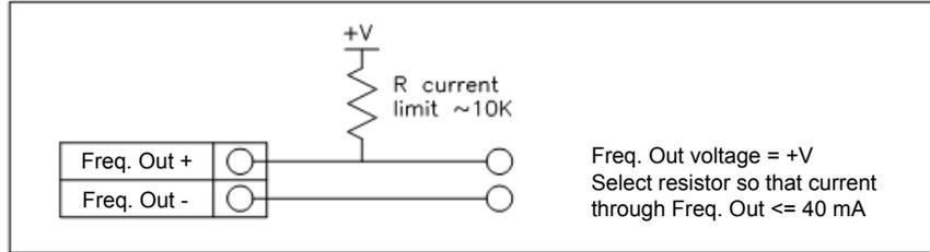
Figure 21. Isolated Frequency Output Using External Power Supply
