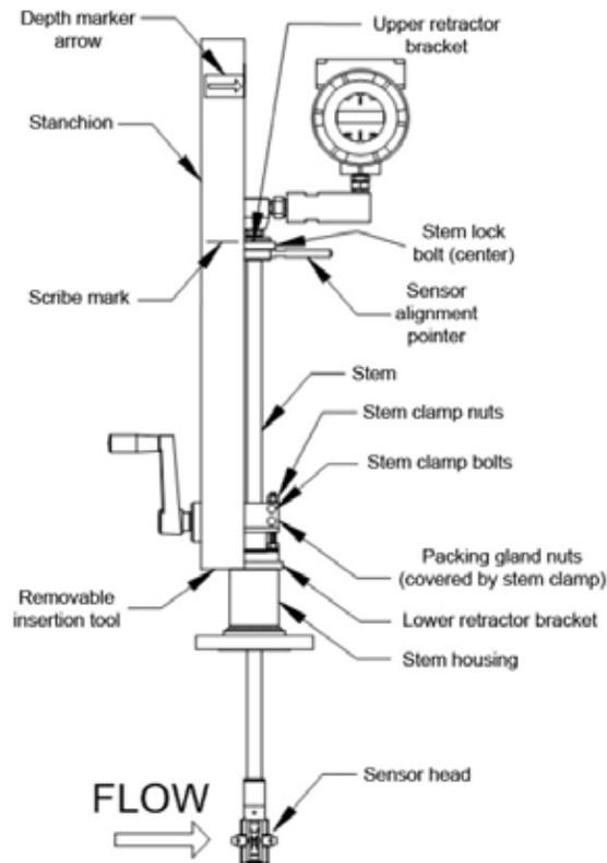
Figure 12. Flow Meter with Removable Insertion Tool
