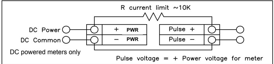
Figure 38. Non-Isolated Pulse Output Using Input Power Supply
