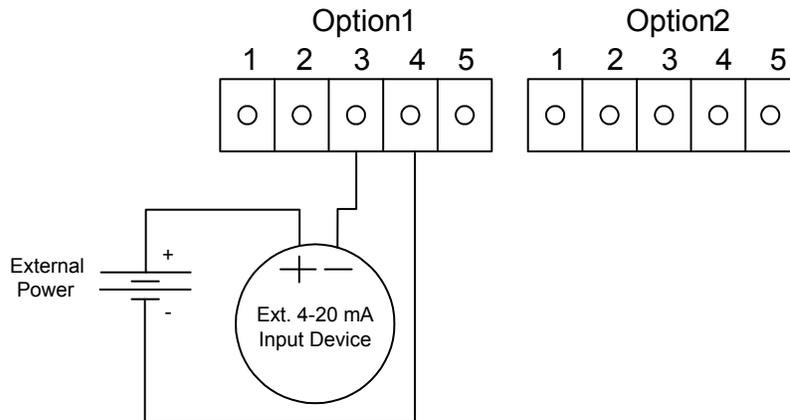
Figure 45. External 4-20 mA Input Wiring - External Power Supply
