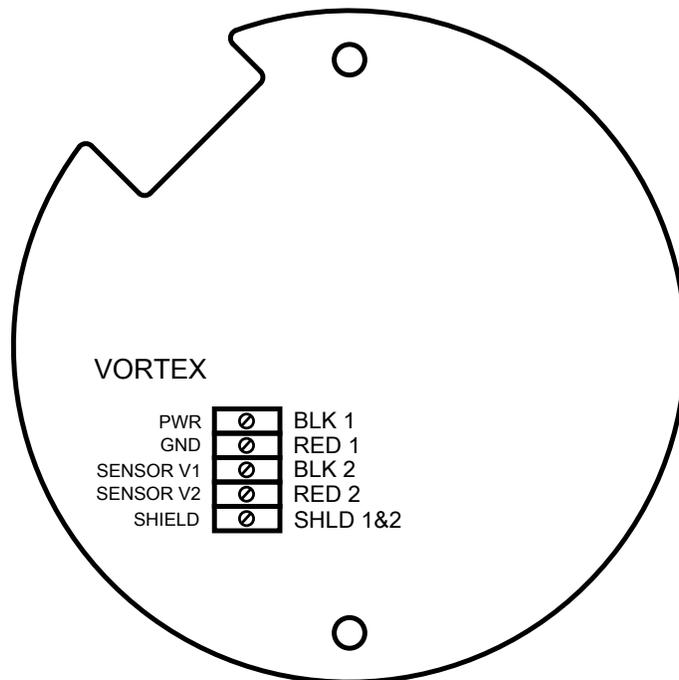
Figure 24. Loop-Powered Volumetric Flowmeter Junction Box Sensor Connections
