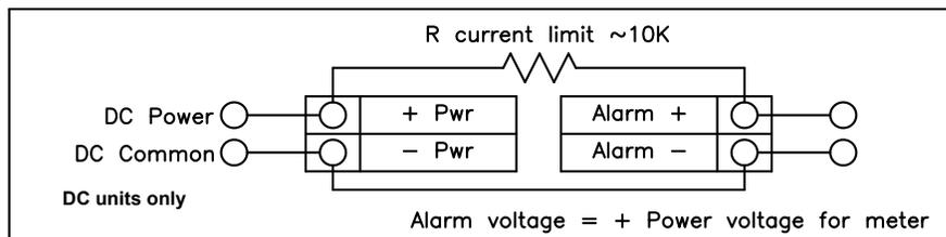
Figure 41. Non-Isolated Alarm Output Using Internal Power Supply
