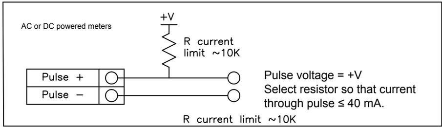
Figure 37. Isolated Pulse Output Using External Power Supply
