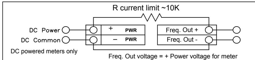
Figure 35. Non-Isolated Frequency Output Using Input Power Supply
