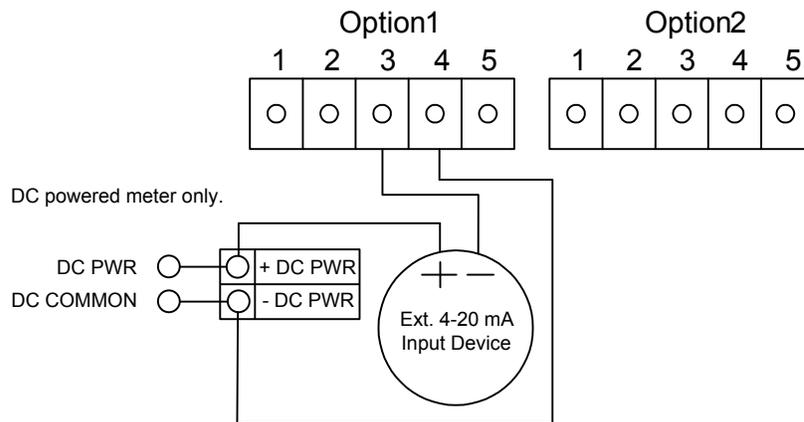
Figure 46. External 4-20 mA Input Wiring - DC Powered Meter
