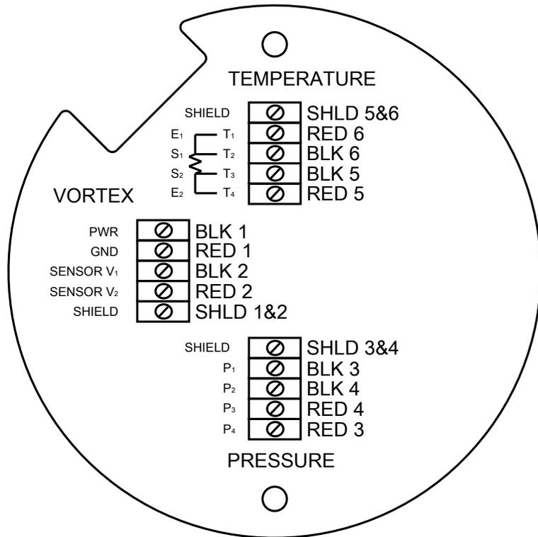
Figure 25. Loop-Power Mass Flowmeter Junction Box Sensor Connections
