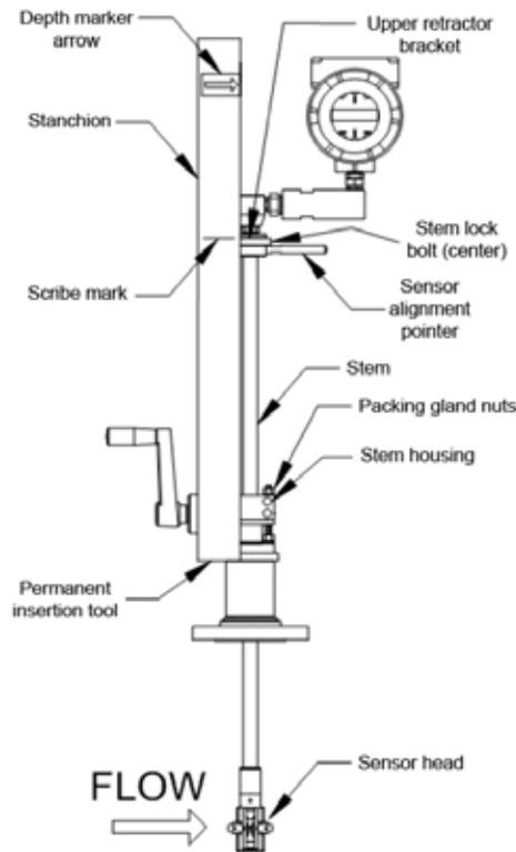
Figure 11. Flow Meter with Permanent Insertion Tool
