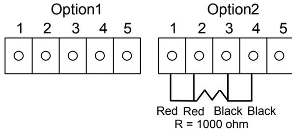
Figure 44. Optional Energy EMS RTD Input Wiring
