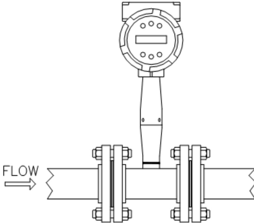
*Figure 1. In-Line Multi-Parameter Vortex Mass Flow Meter*
