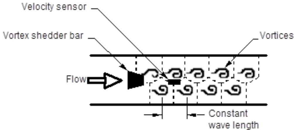
Figure 2. Measurement Principle of Vortex Flow Meters
