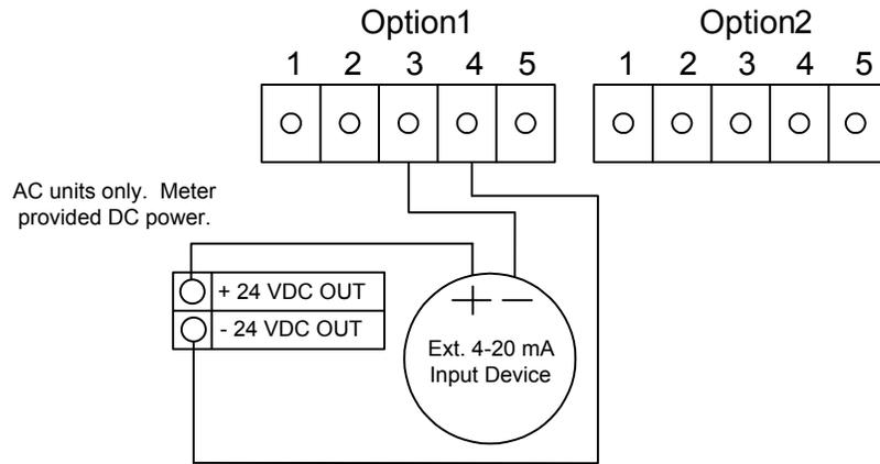
Figure 47. External 4-20 mA Input Wiring - AC Powered Meter
