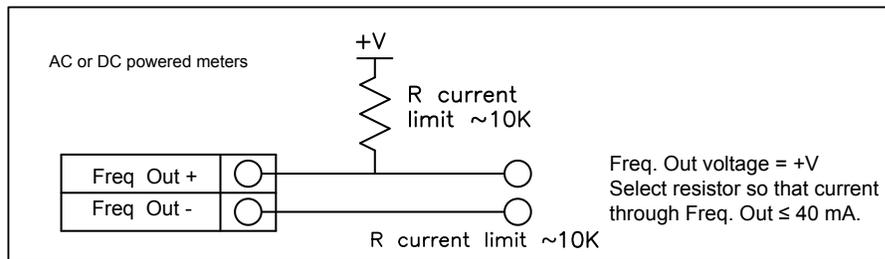
Figure 34. Isolated Frequency Output Using External Power Supply
