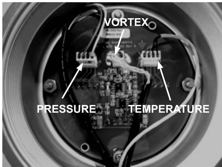
*Figure 55. Remote Feed Through Board Sensor Connections*
