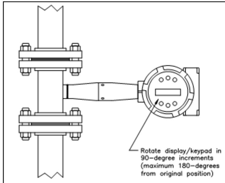
Figure 14. Display/Keypad Viewing Adjustment
