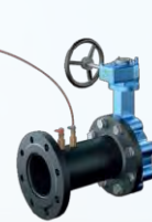
Flanged cast iron pressure differential balancing valves Size: DN40 ~ DN250 | Body: Cast iron Pressure: PN16 | Temperature: -10°C ~ 120°C
