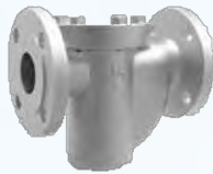
Flanged cast iron strainers Size: DN20 ~ DN200 | Body: Cast iron (GC200) Maximum pressure: 1.0 MPa | Temperature: <120°C
