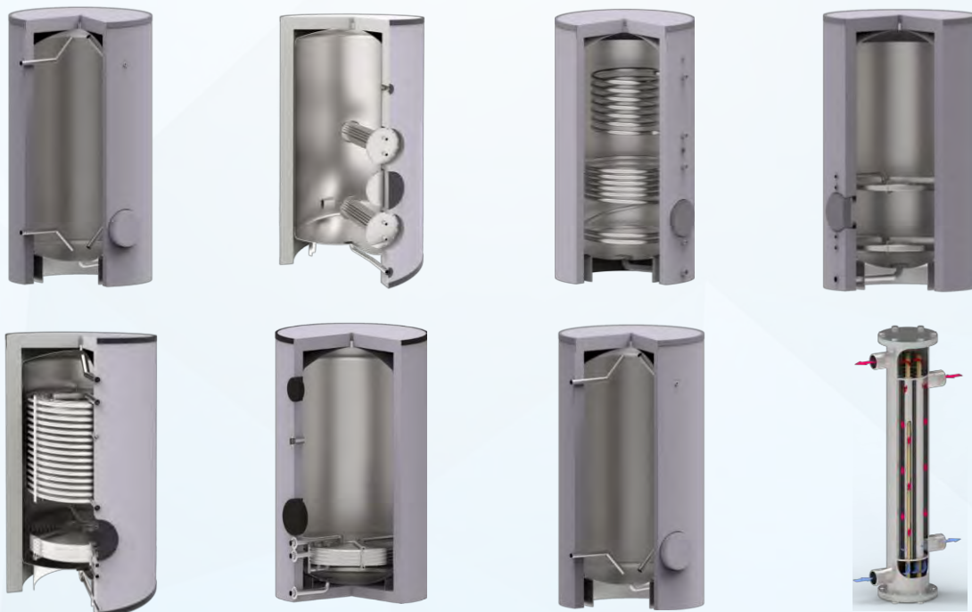
STORAGE WATER HEATER WITH INTEGRATED FLAT COIL HEAT EXCHANGER | STORAGE WATER HEATER | UNIVERSAL WATER HEATER Pressurized thermal storage tank | Pressurized thermal storage tank with the Stainless steel heating coil Capacity 200L ~ 20.000L | Body material: High-quality Stainless steel 316 | Maximum dynamic pressure: 10 bar
