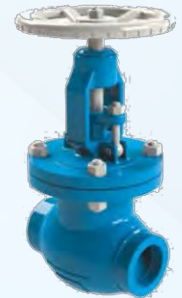
Flanged/welded globe valve Size: 50A – 600A Body: Carbon Steel/ Stainless Steel/ Alloy Steel Working pressure: Class 150 – 1500 Maximum working temperature: +538°C
