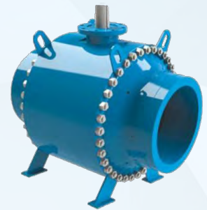
Bolted body ball valve, flanged/welded Size: DN15 – DN1400 | Body: Carbon Steel/ Alloy Steel/ Stainless Steel Working pressure: PN16 – PN326 Working temperature: -50°C ~ +200°C
