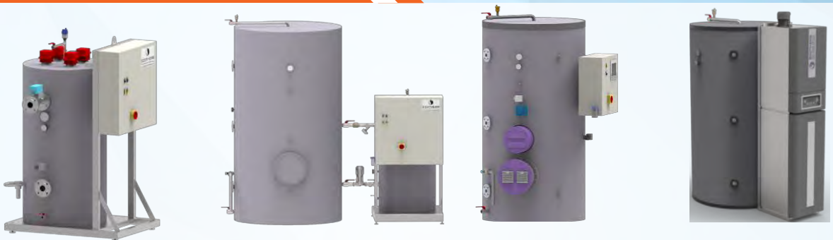
DIRECT/INDIRECT FIRED WATER HEATER (WITH COMPACT GAS CONDENSING BOILER) Direct heating tank use a compact gas condensing boiler | Indirect heating tank uses the heat exchanger suitable for hard water Direct heating tank uses the ceramic heating component | Direct heating tank uses the incology heating component Capacity 300L ~ 10.000L | Body material: High-quality Stainless steel 316
