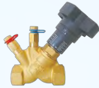
Threaded manual balancing valves Size: DN15 ~ DN50 | Body: Bronze Pressure: PN16/PN25 | Temperature: -10°C ~ 220°C
