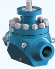
Top-entry soft sealed ball valve Size: DN15 – DN1400 | Body: Carbon Steel/ Alloy Steel/ Stainless Steel Working pressure: PN16 – PN326 Working temperature: -50°C ~ +200°C
