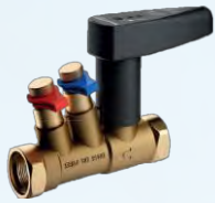
Threaded manual balancing valves Size: DN15 ~ DN50 | Body: Bronze Pressure: PN16/PN25 | Temperature: -10°C ~ 220°C
