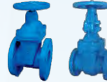
Ductile iron gate valves - rising/non-rising stem, flanged end Pressure: PN16/PN25 | Temperature: -10°C - 120°C
