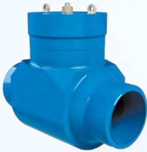
Swing check valve with pressure seal bonnet Size: DN100 – DN300 | Body: Carbon Steel/ Austenite Steel Maximum working pressure: 20Mpa Working temperature: -50°C ~ +350°C
