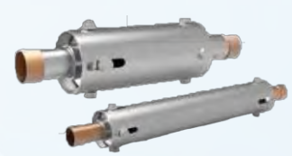
Welded stainless steel expansion connector Size: DN25 ~ DN200 | Body: Stainless steel (STS) Maximum pressure: 1.0 MPa | Temperature: <220°C
