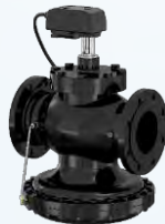
Flanged PICV Body: Cast iron | Control: Modulating/ On-Off Pressure: PN16 | Temperature: 5°C ~ 120°C
