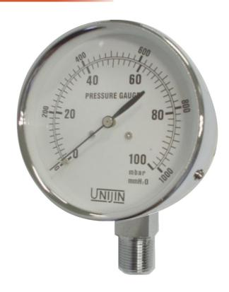
P421 models are designed for non-corrosive environment with extremely sensitive and accurate. The brass chamber element is designed to measure low pressure, compound and vacuum for gaseous and dry air media from as low as 30mbar. P421 model is complete with external zero adjustment screw at its back case for easy re-calibration when necessary.
