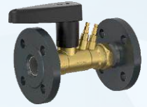
Flanged cast iron manual balancing valves Size: DN50 ~ DN600 | Body: Cast iron Pressure: PN16/PN25 | Temperature: -20°C ~ 120°C
