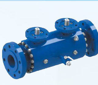
Double block and bleed valve Size: DN15 ~ DN1400 | Body: Carbon Steel/ Alloy Steel/ Stainless Steel Working pressure: PN16 ~ PN326 Working temperature: -50°C ~ +200°C
