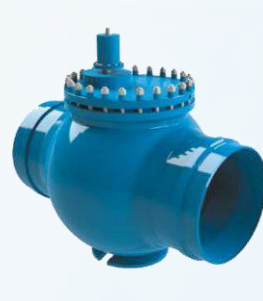
Welded swing check valve with remote indication of stop device position Size: DN80 ~ DN600 Body: Carbon Steel Working pressure: 20 MPa Maximum working temperature: +350°C
