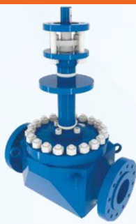
Top-entry cryogenic ball valve Size: DN15 ~ DN500 | Body: Carbon Steel/ Alloy Steel/ Stainless Steel Working pressure: PN16 ~ PN326 | Working temperature: -50°C ~ +200°C
