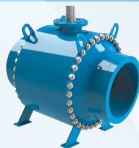
Bolted body ball valve, flanged/welded Size: DN15 ~ DN1400 | Body: Carbon Steel/ Alloy Steel/ Stainless Steel Working pressure: PN16 ~ PN326 Working temperature: -50°C ~ +200°C
