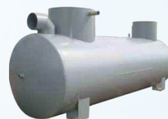
Cylindrical oil separator with sludge trap and coalescing filter, size 30 - 50 l/s
