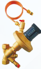
Threaded bronze pressure differential balancing valves Size: DN15 ~ DN50 | Body: Brass / Cast iron Pressure: PN16/PN25 | Temperature: -20°C ~ 120°C
