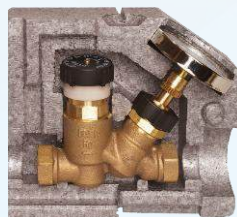
Brass threaded thermal balancing valves Size: DN15, DN20, DN25 | Body: Brass | Pressure: 10Bar/16Bar Temperature range: 40°C ~ 65°C / 40°C ~ 50°C / 50°C ~ 60°C
