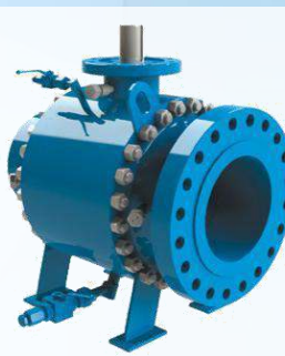
Metal seated ball valves, welded/flanged Size: DN15 ~ DN1400 | Body: Carbon Steel/ Alloy Steel/ Stainless Steel Working pressure: Class 150 - 2500 | Working temperature: -50°C ~ +550°C
