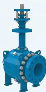
Ball valve Size: 50A ~ 300A Body: Steel (SCPH2) Working pressure: 0.98MPa/1.96MPa Maximum working temperature: 120°C/220°C
