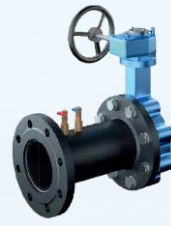
Flanged cast iron manual balancing valves Size: DN50 ~ DN600 | Body: Cast iron Pressure: PN16/PN25 | Temperature: -20°C ~ 120°C
