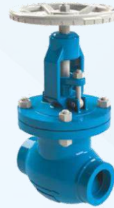
Flanged/welded globe valve Size: 50A ~ 600A Body: Carbon Steel/ Stainless Steel/ Alloy Steel Working pressure: Class 150 - 1500 Maximum working temperature: +538°C
