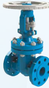
Flanged/welded gate valve Size: 50A ~ 1200A Body: Carbon steel/ Stainless steel/ Alloy steel Working pressure: PN16 ~ PN100 Maximum working temperature: +538°C
