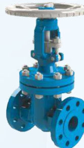
Flanged/welded gate valve Size: 50A – 1200A Body: Carbon steel/ Stainless steel/ Alloy steel Working pressure: PN16 – PN100 Maximum working temperature: +538°C
