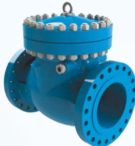
Swing check valve Size: DN15 – DN1050 | Body: Carbon Steel/ Alloy Steel/ Stainless Steel Working pressure: PN16 – PN326 | Working temperature: -50°C ~>200°C
