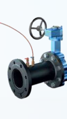
Flanged cast iron pressure differential balancing valves Size: DN40 ~ DN250 | Body: Cast iron Pressure: PN16 | Temperature: -10°C ~ 120°C
