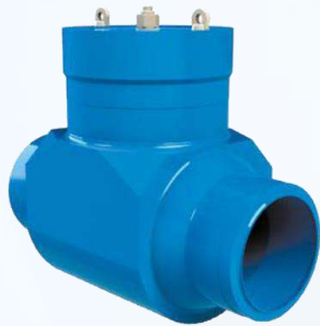
Swing check valve with pressure seal bonnet Size: DN100 – DN300 | Body: Carbon Steel/ Austenite Steel Maximum working pressure: 20Mpa Working temperature: -50°C ~ +350°C
