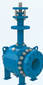
Ball valve Size: 50A – 300A Body: Steel (SCPH2) Working pressure: 0.98MPa/1.96MPa Maximum working temperature: 120°C/220°C
