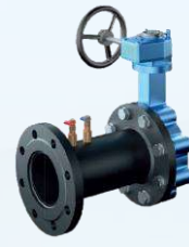
Flanged cast iron manual balancing valves Size: DN50 ~ DN600 | Body: Cast iron Pressure: PN16/PN25 | Temperature: -20°C ~ 120°C
