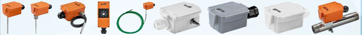
TEMPERATURE SENSORS FOR WATER AND AIR SYSTEMS Temperature sensor | Measurement range : 50°C ~ 250°C (optional) | Output signal: switch type, PT100, PT1000, NI1000, NI1000IK5000, NTC10K2, NTC10K, NTC20K, NTC10K3, 0 - 5V, 0 - 10V, 4 - 20mA
