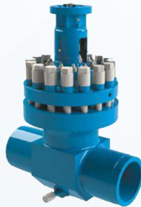
Welded gate valve Size: DN50 – DN800 Body: Carbon Steel/ Austenite Steel Maximum working pressure: 20Mpa Maximum working temperature: +350°C
