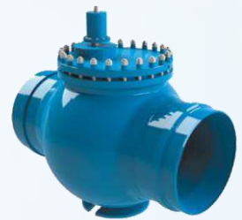
Welded swing check valve with remote indication of stop device position Size: DN80 – DN600 Body: Carbon Steel Working pressure: 20 Mpa Maximum working temperature: +350°C
