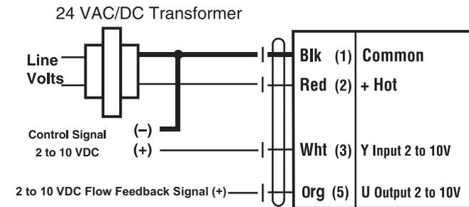
2 to 10 VDC control signal for Non-Spring Return and Electronic Fail-Safe
