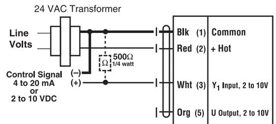
4 to 20 mA control signal for Non-Spring Return and Electronic Fail-Safe
