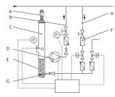
For deaerating the water, the system water is drawn in via a bypass from the return line of the system (H). The water is run through a flow regulator (G) and the strainer (F) into the deaeration tank (C). It is subjected to a vacuum during the cyclic running of the pump (D) and passed through a Pall-ring (E). As a result of the lowered pressure, and the large surface of the Pall-ring, air dissoleves from the water.
