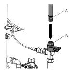
Connect the supply line of the system to the pressure side of the ENA
