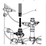
Connect the return line of the system to the inlet of the ENA.
