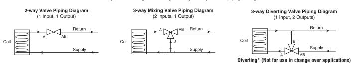
The BELIMO Characterized Control Valve is a CONTROL valve, not a manual valve adapted for actuation. The control port is the A-port. It is similar to the globe valve in that the middle port is the B or bypass port. The common port AB is on the main opposite the A-port. These diagrams are for typical applications only. Consult engineering specification and drawings for particular circumstances.
