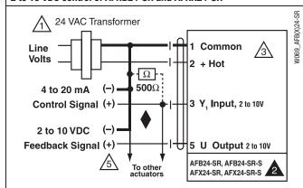
4 to 20 mA control of AFRB24-SR and AFRX24-SR with 2 to 10 VDC feedback output
